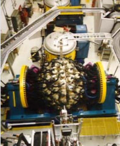
View of the gamma detector array GAMMASPHERE which was used in the experiment described below. It consists of about 100 Ge crystals used for the high-resolution detection of gamma rays from nuclear reactions.
